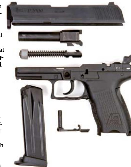
The P2000 quickly field strips into six basic sub-assemblies for cleaning and maintenance. Note the polymer recoil bushing on the front of the steel guide rod for the recoil spring.
